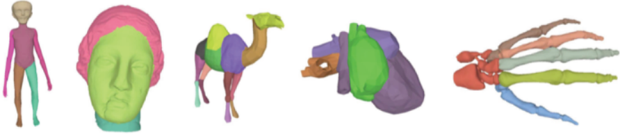
Figure 1.11. Segmentation based on membership probabilities. Image from [KAT 03]. For a color version of this figure, see www.iste.co.uk/mari/analysis.zip
