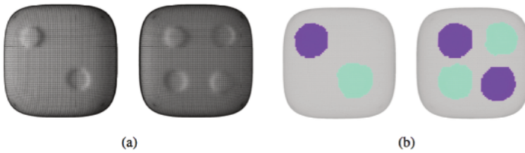
Figure 1.23. Feature detection between two meshes: (a) input meshes and (b) extracted features. For a color version of this figure, see www.iste.co.uk/mari/analysis.zip
