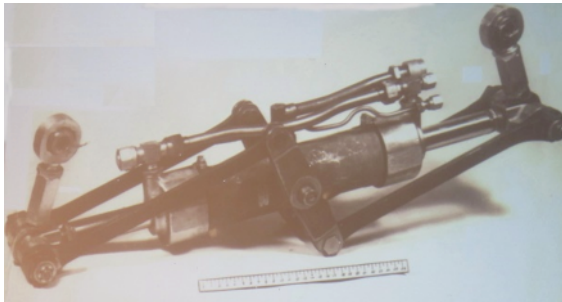
Figure 1.15. Missile wing deployment mechanism (source: Christian Lardier)
