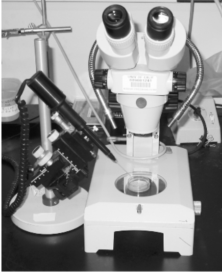
Fig. 1.1 Apparatus for cytoplasmic injection of Xenopus oocytes. The oocytes are distributed on polypropylene mesh in a 35-mm tissue culture dish on the stage of a dissecting microscope. Injection needles are made using a pipette puller to draw out the glass bores that are normally used with the microdispenser. After pulling, the needles are broken off at a tip diameter of 20–40 \mu\text{m} , as measured with a reticle under a dissecting microscope. The injection needle is position over individual oocytes using a micromanipulator and the oocytes are injected with up to 100 nl of RNA solution. Using these procedures, it is possible to inject 20 oocytes with one sample in a few minutes.
